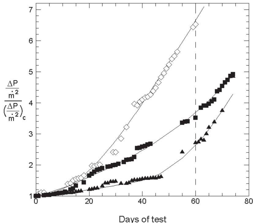
Figure 7. Hydrodynamic criterion for assessing the antifouling device. Open symbols denote data with the antifouling device switched off;  $\blacktriangle$  denote data with the antifouling device installed in line with the flow (EAF-1) and  $\blacksquare$  data with the device not in line with the flow (EAF-2).
