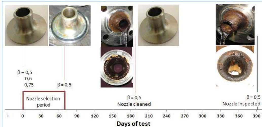
Figure 6: Sensitivity of the flow measuring device to biofouling formation
