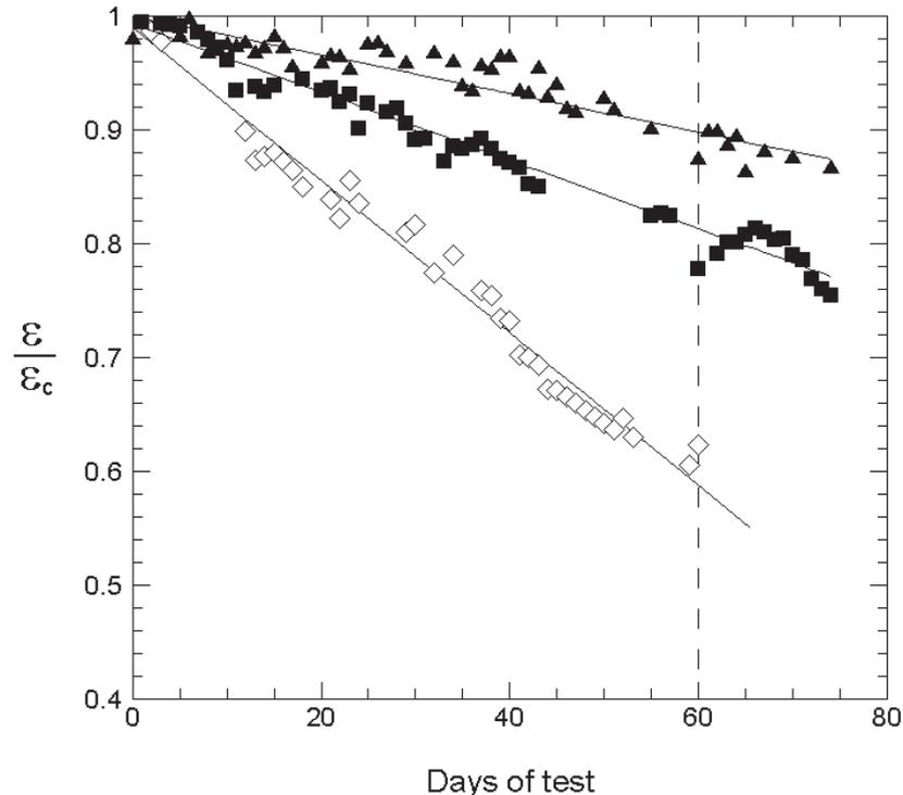
Figure 8. Thermal criterion for assessing the antifouling device. Open symbols denote data with the antifouling device switched off; ▲ denote data with the antifouling device installed in line with the flow (EAF-1) and ■ data with the device not in line with the flow (EAF-2).
