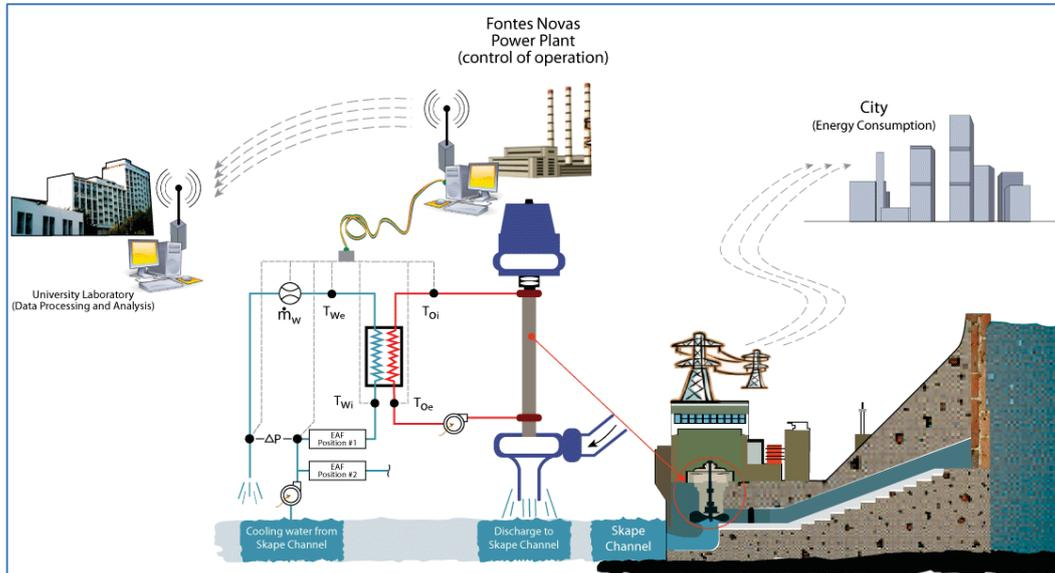
Figure 4 schematic picture of the cooling system of the journal bearings of the turbines and the remote data acquisition/transmitter web-based system. (EAF-1: antifouling device installed in line with the flow; EAF-2: antifouling device not in line with the flow).
