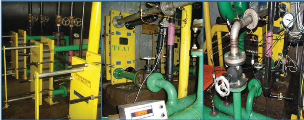
Figure 5: The instrumented (vertical plate) heat exchangers and the flow rate measuring system
