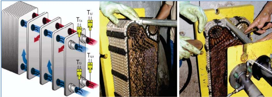
Figure 3. Biofouling formation in plate heat exchanger (2-a: overall schematic; 2-b: fouled plates after exposed to the flow).
